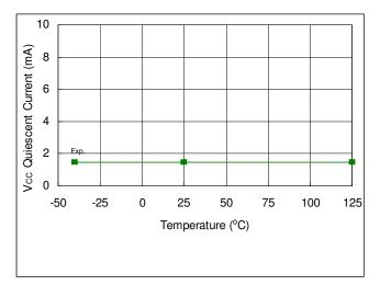
Fig. 28. V<sub>CC</sub> Quiescent Supply Current vs. Temperature
