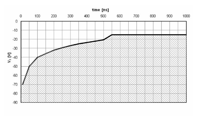
Figure 18: Negative V<sub>S</sub> transient SOA for IRS2608D @ VBS=15V
