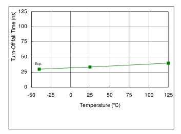
Fig. 25. Turn-off Rise Time vs. Temperature
