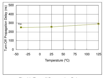
Fig. 23. Turn-off Propagation Delay vs. Temperature
