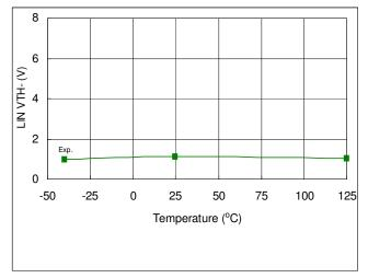
Fig. 38. LIN  $V_{\text{TH-}}$  vs. Temperature
