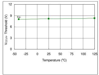
Fig. 31. V<sub>CCUV-</sub> Threshold vs. Temperature
