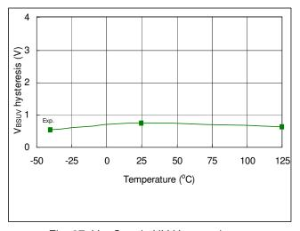
$\begin{array}{c} \text{Fig. 27. V}_{\text{BS}} \text{ Supply UV Hysteresis vs.} \\ \text{ Temperature} \end{array}$
