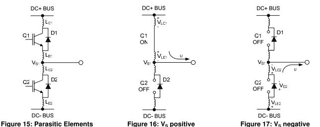
In a typical motor drive system, dV/dt is typically designed to be in the range of 3-5 V/ns. The negative  $V_S$  transient voltage can exceed this range during some events such as short circuit and over-current shutdown, when di/dt is greater than in normal operation.
