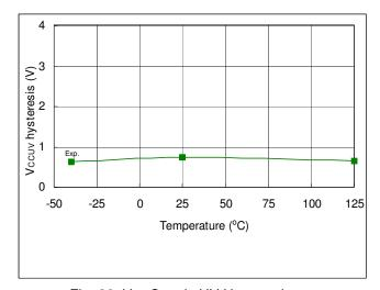
Fig. 26.  $V_{CC}$  Supply UV Hysteresis vs. Temperature
