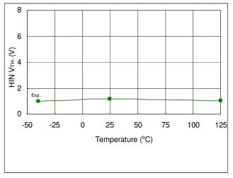
Fig. 40. HIN  $V_{\text{TH-}}$  vs. Temperature
