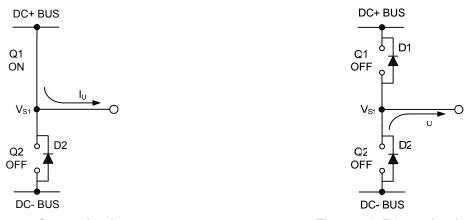
Figure 11: Q1 conducting
