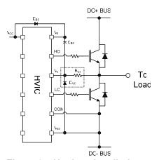
Figure 21: V<sub>S</sub> clamping diode
