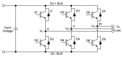
Figure 10: Three phase inverter
