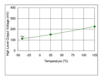
Fig. 35. High Level Output Voltage vs. Temperature
