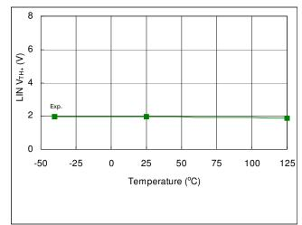
Fig. 37. LIN V<sub>TH+</sub> vs. Temperature
