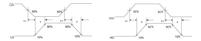
Figure 3: Switching time waveforms
