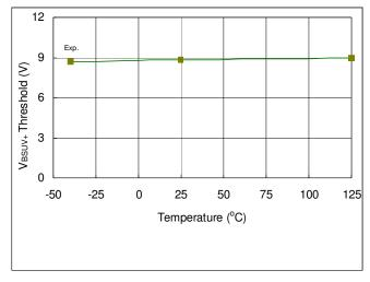
Fig. 32. V<sub>BSUV+</sub> Threshold vs. Temperature
