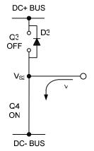
Figure 13: D3 conducting
