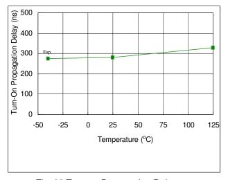
Fig. 22 Turn-on Propagation Delay vs. Temperature
