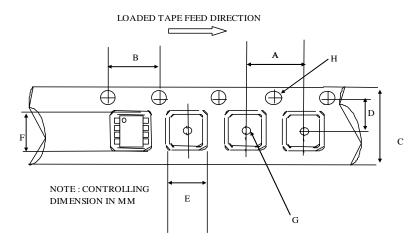
CARRIER TAPE DIMENSION FOR 8SOICN
