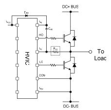
Figure 20: V<sub>S</sub> resistor
