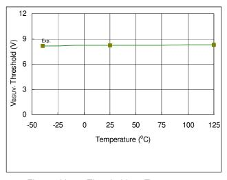
Fig. 33.  $V_{\text{BSUV}}$ . Threshold vs. Temperature
