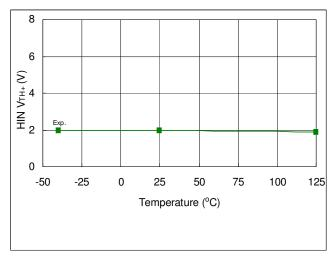
Fig. 39. HIN  $V_{TH_+}$  vs. Temperature
