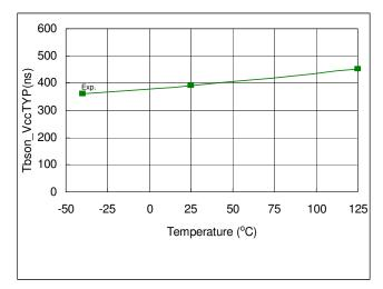
Fig. 41. Tbson\_ $V_{CC}TYP$  vs. Temperature
