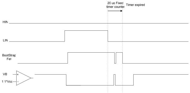
Figure 9: BootFET timing diagram
