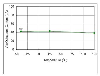
Fig. 29  $V_{BS}$  Quiescent Supply Current vs. Temperature
