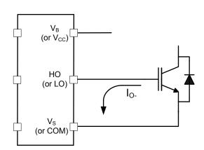
Figure 2: HVIC sinking current
