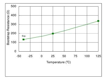
Fig. 36. Bootstrap Resistance vs. Temperature
